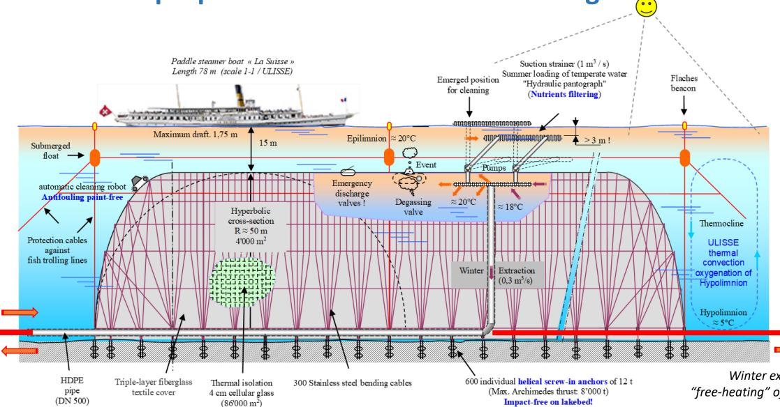
Typical ULISSE reservoir: hemi-cylindrical dimensions:  $550 \times 100 \times 50 \text{ m}$ , volume 2'000'000 m<sup>3</sup> Energy content: 125 TJ @  $\Delta T$  15 K  $\approx$  2'900 toe, avoid 9'600 t  $CO_2$
