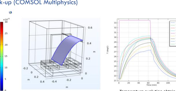
Convection Velocity scale (mm/s) Temperature distribution at end discharging (COMSOL)
