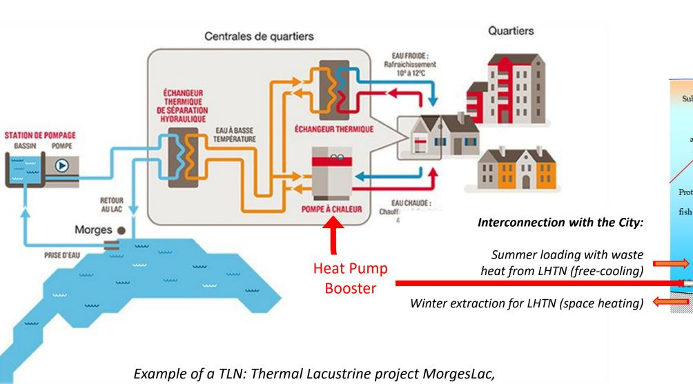
Under Lake Infrastructure for thermal capture and Storage of Solar Energy
